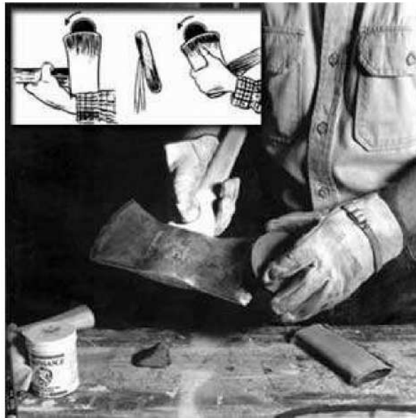
Figure 71--Use the ax stone in a circular motion, working into the edge, toward the middle of the ax head (drawings by Frederic H. Kock).
