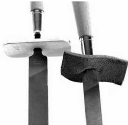
Figure 64--File guards help keep your fingers away from the sharpened ax blade.
